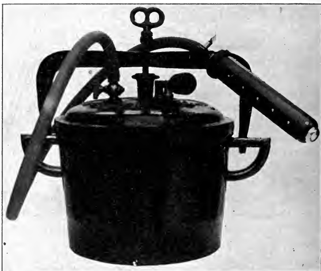
Fig. 71.—Kommerell steam pot with author's insulated handle. The cover of the pot is securely held down by the bar and screw. At the left of the cover is seen the cock for turning the steam into the pipe and handle. To the right is seen a safety-valve. The handle consists of an inner metal tubing capped by a blunt head, in the center of which is a small opening. Around the tubing is an air-space and then the insulated substance, which does not get hot during the passing of steam. The small points seen on the handle are metal tacks to give the hand a better purchase.
